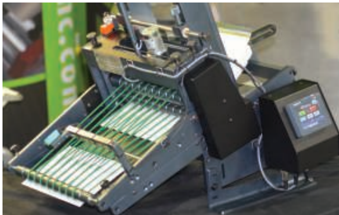
FIGURE 6. Open Source friction feeders from Pineberry Manufacturing include a PLC touchscreen with smartphone app capabilities
