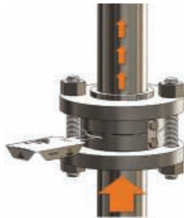
FIGURE 2. Leaks can occur through the relief system if rupture discs become compromised
