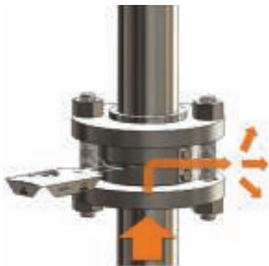
FIGURE 3. Leaks can occur outside of the planned flow path in rupture disc systems if all components are not correctly installed
